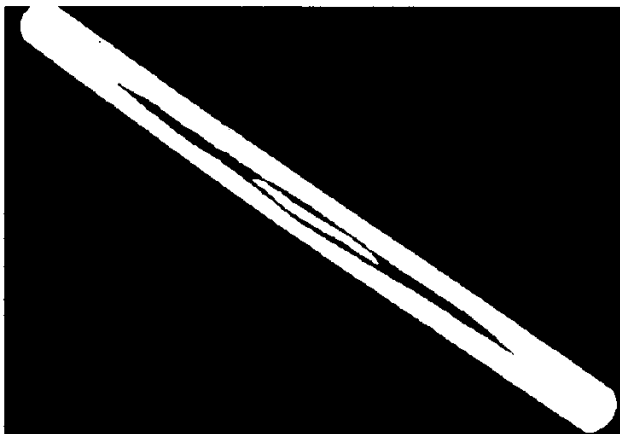
Fig. 1. - Metallographic cross-section of a monofilamentary BSCCO-2223 tape.
